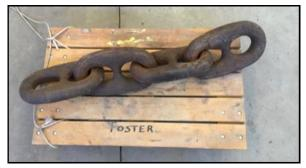
This is "D lock" anchor chain from the SS *Spartan*, sister ship to the *Badger*. Each link weighs 25 lbs. and is probably original to the boat's building in 1952.
