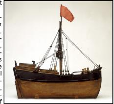
the mast. The ship's bell is located back aft on the transom cap rail. The rudder appears to have a tiller bar that extends into the aft deck shelter, and there are external block and tackle arrangements set up on the quarters that are also fastened to the rudder. There are two deck fit-
