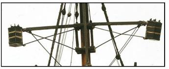
piece built 'bread and butter' style, and gauged out internally. The model is decked, equipped and rigged with two lanterns suspended from a yard that is square in cross section that could be raised and lowered during times of use. The yard is attached to a structure that can slide up and down the mast. The mast itself is one massive piece
